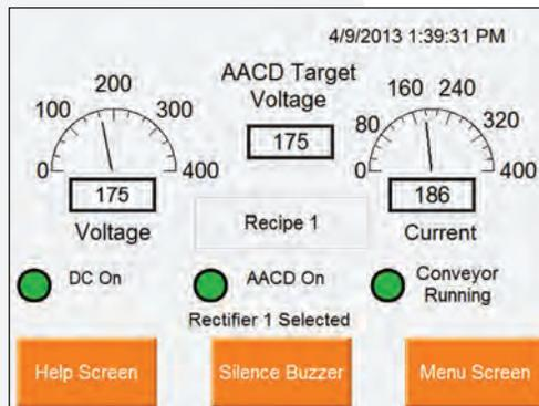
"Monitoring & Status" screen includes output voltage and current measurements, as well as verification that the target voltage is met.
