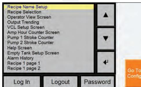
"Main Menu" screen includes access to all operational data, programming, status, and alarm logs.
