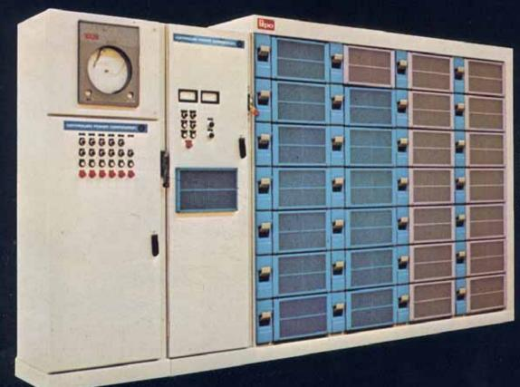
Expandable from 900 Amps. to over 2,000 Amps. this, 500 KVA system for electrocoating also incorporates complete process control instrumentation in an integral cabinet.
