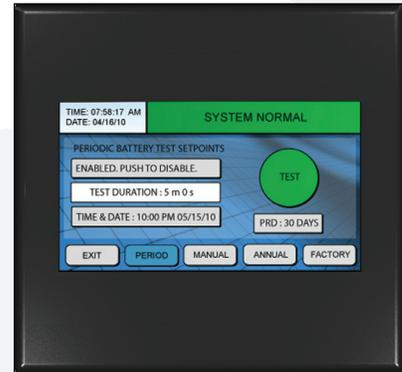
The color touchscreen display on the **Intellistat TS** provides all electrical parameters, inverter status, programmable inverter and battery testing, and data-logging. Optional **Intellistat TS** communications allow for remote monitoring and reporting. For more details, see the “Optional Network Communications” description on Page 7.
