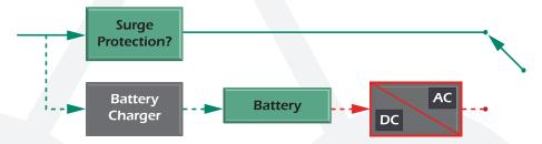
System performance is verified under only two conditions: 1) if / when it is periodically tested, and 2) during an emergency. MAY NOT provide surge protection, and DOES NOT provide power conditioning or regulated voltage to LED drivers and electronic ballasts that are being utilized for egress lighting. Inverters promoting 98+ % efficiency are typically off-line or standby designs, or "operating" in a bypass / standby mode.
